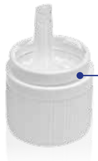
KG KPV OVII NW18 Child-resistant tamper-evident vertical dropper closure Material: Outer cap PE-HD; Inner cap PE-HD; Dropper PE-LD Thread: DIN 168 GL 18
