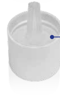
KG KPV SMOOTH NW18 Child-resistant vertical dropper closure; variant "smooth" Material: Outer cap POM; Inner cap PP; Dropper PE-LD Thread: DIN 168 GL 18
