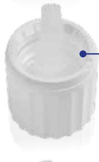
KPV OVIII 20 NW18 Tamper-evident vertical dropper closure; variant 20 Material: Cap PP; Ring PE-HD; Dropper PE-LD Thread: DIN 168 GL 18
