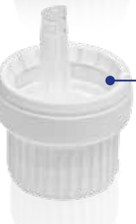
KPV OVIII NW18 Two-part tamper-evident vertical dropper closure Material: Cap PP; Tamper-evident band PE-HD; Dropper PE-LD Thread: DIN 168 GL 18
