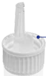
KPV NW18 Standard vertical dropper closure Material: Cap PP; Dropper PE-LD Thread: DIN 168 GL 18
