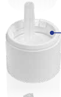
KPV OVIII DW NW18 Two-part tamper-evident vertical dropper closure; DW variant Material: Cap PP; Tamper-evident band PE-HD; Dropper PE-LD Thread: DIN 168 GL 18
