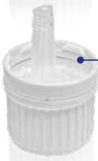
KPV OVII NW18 Child-resistant tamper-evident vertical dropper closure Material: Outer cap PE-HD; Inner cap PE-HD; Dropper PE-LD Thread: DIN 168 GL 18
