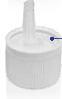
KG KPV NW18 Child-resistant vertical dropper closure Material: Outer cap PE-HD; Inner cap PP; Dropper PE-LD Thread: DIN 168 GL 18
