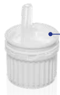
KPV OVII (PP) NW18 Child-resistant tamper-evident vertical dropper closure Material: Outer cap PE-HD; Inner cap PE-HD; Dropper PE-LD Thread: DIN 168 GL 18
