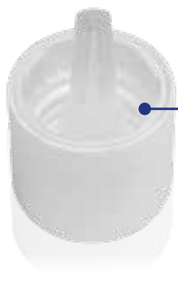
KG KPV OVII SMOOTH NW18 Child-resistant vertical dropper closure; variant "smooth" Material: Outer cap PP; Inner cap PE-HD; Dropper PE-LD Thread: DIN 168 GL 18
